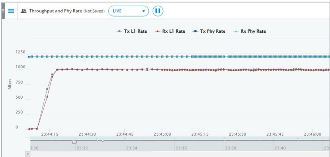
UDP Throughput Performance Example showing 2x2 MIMO, 1518-byte, Time Series from Spirent TestCenter IQ
