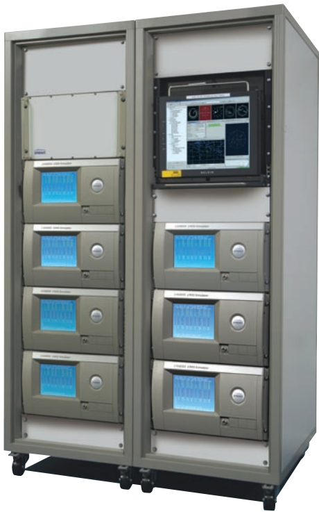
Spirent GSS8000 7 element CRPA test system
